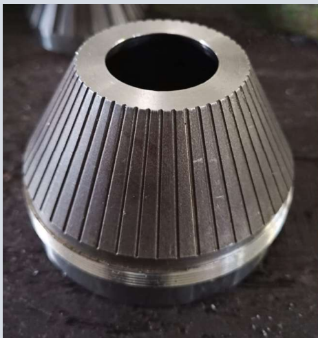
Manufactured Powder Delivery nozzle for metal 3D printer
