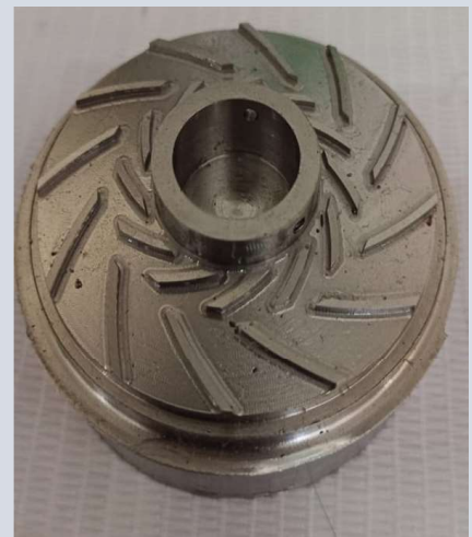
Manufactured Powder Delivery nozzle for metal 3D printer
