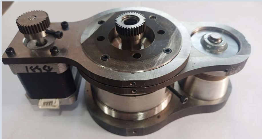
Manufactured Powder Delivery nozzle for metal 3D printer
