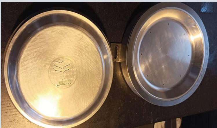
Compression Mould for Eco-friendly Areca nut leaf plate
